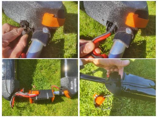
8) Lift the motor part and place the sled into the two designated holes at the bottom of the motor part. Secure the Velcro tightly around the sled attachment.
