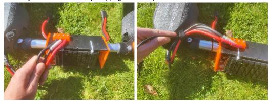
7) Plug the 2 cables from the controller into the battery.
