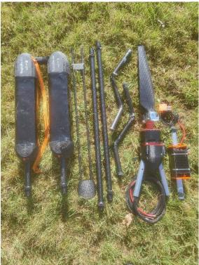
1) Route the motor cables through the tube. Attach the carbon tubes to the motor part and insert the Velcro strip with the aluminum plug into the corresponding holes. Ensure everything is securely fastened.
