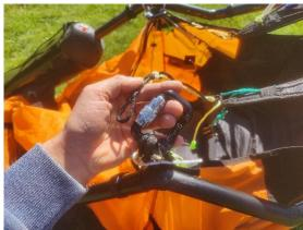
10) Hook the aluminum frame into the carabiner, place the loop over the aluminum frame, and then loop it back over the carabiner.
