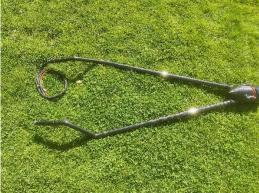
3) Pull the motor cable through the carbon tube of the battery and slide the rear of the battery tube over the aluminum. Insert the Velcro strip with the plug into the corresponding holes and ensure everything is securely fastened.
